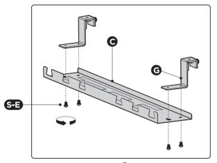
Attach the **tray hangers** to the cable **management tray** with **4 screws S-E** from below using a **Phillips screwdriver**.
