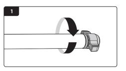
• Turn the knob as shown to loosen the right side of the **sync rod B** .
