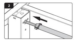
Insert the left end of the sync rod into the column then tighten.
