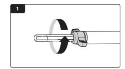
With the frame positioned upright, turn the knob as shown to loosen the left side of the **sync rod B** .
